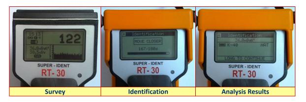
The RT-30 uses an advanced method of Automatic Stabilisation on Natural Background Radiation throughout its operation. This unique method eliminates the need for an additional radioactive check source.
