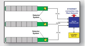
The RS-725 Controller is connected directly to the Plant Network via the Ethernet port giving the RSO direct access to alarm data.
