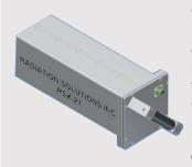
The **RS-725/21** system is a 3"x3" (21 cu ins) Sodium-lodide detector mounted in a square housing. Normally the face of the detector is mounted as close as possible (4-6") from the measurement point and installed in a 1" steel collimator during installation. This collimator reduces local
