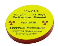
Alpha disk sources is designed for use as reference sources. The radioactive material is chemically plated on to the surface of a silver disk that is mounted at the bottom of the well of a Plexiglas® disk. The completed sources are unsealed and offered in two sizes: 1.0" x 0.125" and 2.0" x 0.125".
