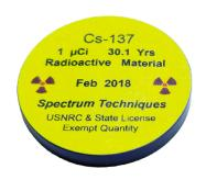
Beta/Gamma disk sources are designed for use as reference sources. The radioactive material is sealed using epoxy in the bottom of the well of a Plexiglas® disk. The completed sources are sealed and offered in two sizes: 1.0" x 0.125" and 2.0" x 0.125".
