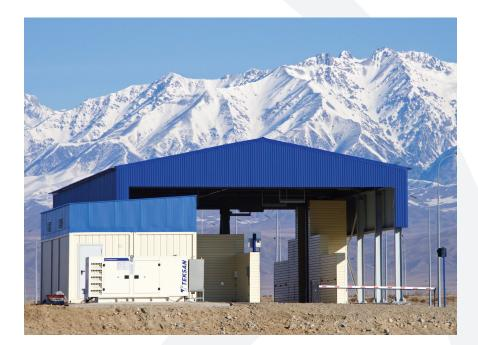
The HXP-FreightScan<sup>™</sup> is a high-energy portal designed for screening trucks and shipping containers at seaports, border crossings, and cargo centers. The portal is fully automated and can process up to 150 trucks an hour. Its precision software allows drivers to remain in their cars during screening and with a tunnel height of almost five meters (16.4 ft.), even oversized cargo can be scanned.
