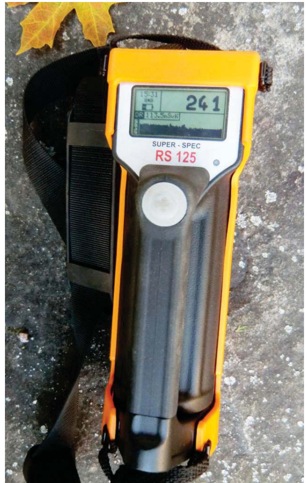
The RS-125 spectrometer comes with a protective boot and a shoulder strap for hands-free surveying
