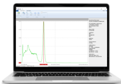
PM1401K-3 Desktop Software for adjusting instrument settings, downloading the operating history and analyzing the gamma spectra
